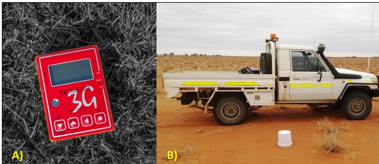
**Figure 3:** Instrumentation and survey acquisition – A) Tromino unit developed to passively measure natural seismic vibrations (courtesy of Resource Potentials Pty Ltd), B) survey method employed at Honeymoon.
