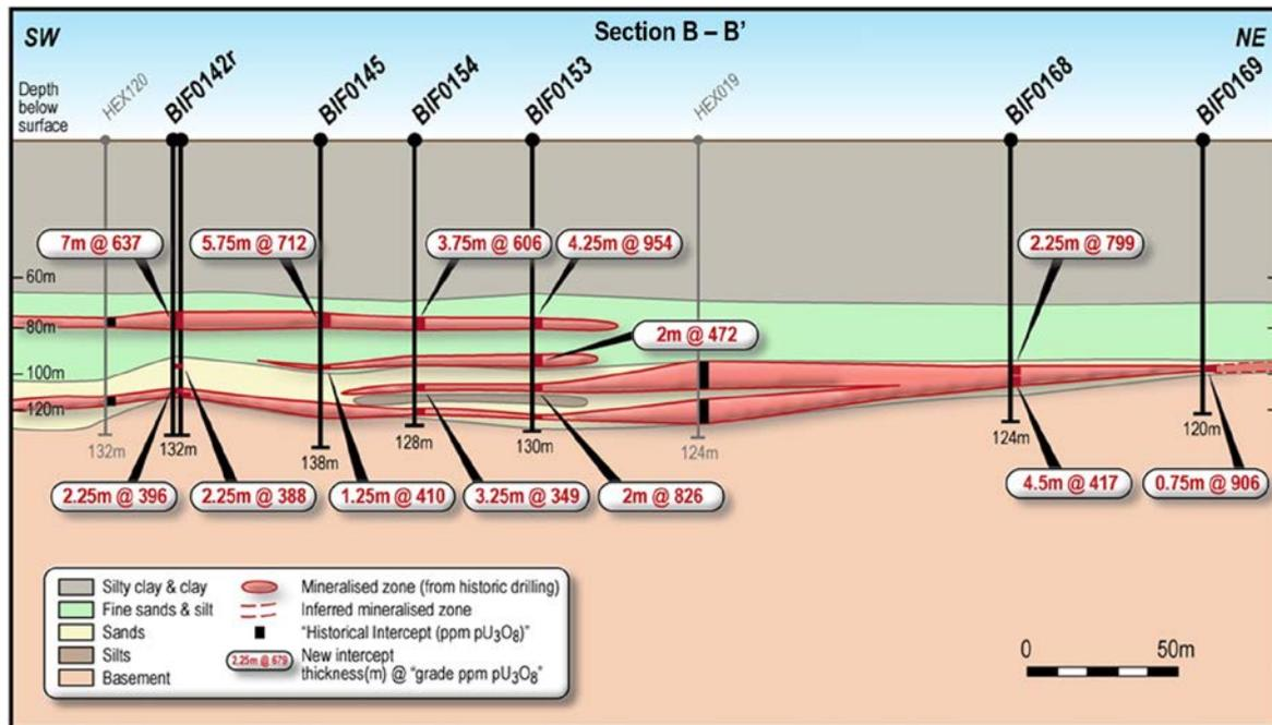
Figure 5: Cross-sectional view from the East Kalkaroo Deposit, showing selected mineralised intercepts.
