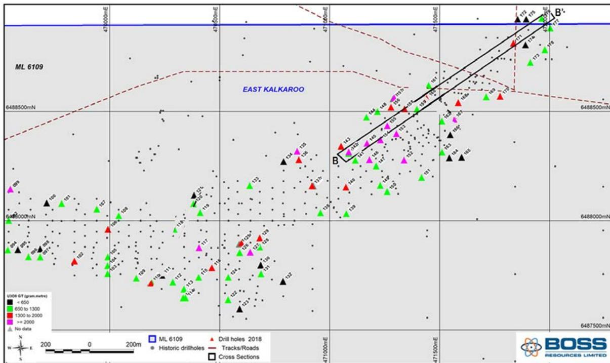
Figure 4: Grade-thickness distribution map for the East Kalkaroo Deposit
