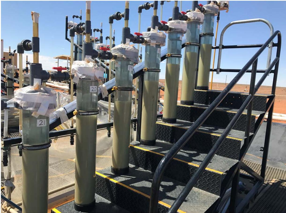
*Figure 2: IX Pilot Plant Loading Columns*
