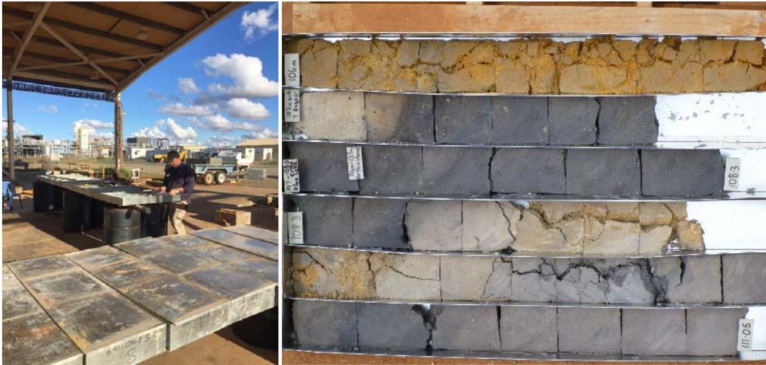
Figure 1: Logging and Sampling of Sonic Core - Holes HMI063S and HEX019S shown.
