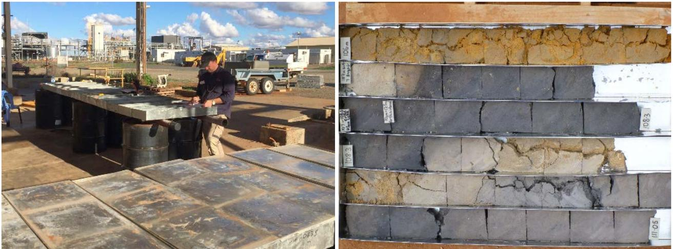
**Figure 1:** Logging and Sampling of Sonic Core - Holes HMI063S and HEX019S shown
