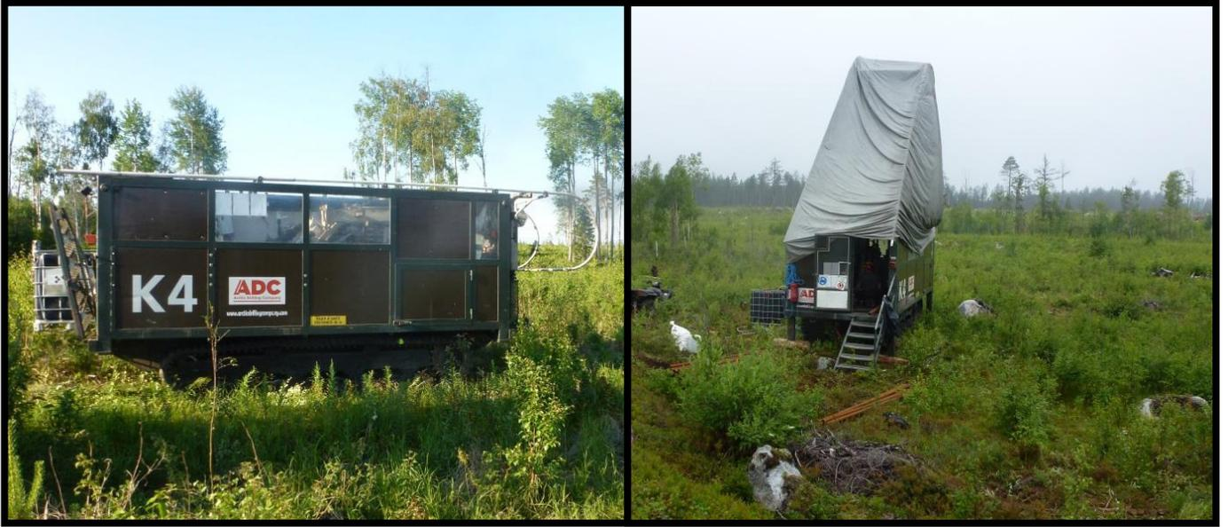
Figures 1 and 2. Small track diamond drill rig being utilised by Boss Resources for the current drill program with minimal footprint and impact on the surrounding environment.
